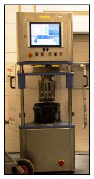
• Contec viscometer for Micro-mortar (Viscometer 6) - for mortar and paste (Dmax  $\leq$  5 mm)
