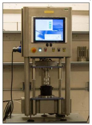
• Rheometer for paste (Modular compact rheometer (MCR) 302) - modular compact rheometer, allows integration of a wide range of temperature devices and application specific accessories. The EC motor technique, the low friction bearing and the patented normal force sensor have been optimized enabling any type or combination of rheological tests, both in rotational and oscillatory mode.
