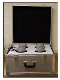
• <u>Calmetrix P-Cal 1000</u> - The P-Cal is a high performance semi-adiabatic calorimeter with high efficiency insulation to achieve close to adiabatic conditions. The P-Cal is the only high performance semi-adiabatic calorimeter that is so portable it can easily be carried in concrete delivery trucks or other field applications. Don't be fooled by its size: the quality of the insulation gives the P-Cal 1000 laboratory-level quality, with precise and replicable measurements.
