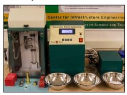
• Gyratory compactor ICT-100R - this piece of equipment is used to test compactability of aggregate and low workable concrete. This model is the most complete equipped version for all kind of laboratory compacting work (research, mix design, specimen preparation etc.).
