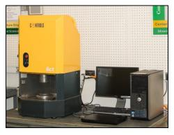
• Mercury intrusion porosimeter (MIP) - Non-wetting fluid (mercury) Intrusion device, by pressure, for pore size distribution determining in solid porous sample. Mercury intrusion pressure is raised automatically, up to 220 MPa, and intruded volume into sample is related with porosity determination. The measuring range of pores is between 7 nm and 0.4 mm.
