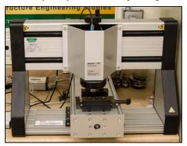
• <u>AVA (Air Void Analyzer)</u> is used to measure the air-void parameters (spacing factor and specific surface) of samples of fresh air-entrained concrete. Samples are taken after concrete has been placed in the structure and consolidated. It provides timely information to reveal problems with the air-void system.
