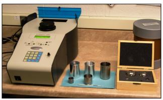
• <u>Blaine Air Permeability</u> - Fineness measurement apparatus: This apparatus is to determine Blaine fineness of powder materials. The Blaine of powder materials has significant influence on workability and rheology of cementitious materials, including concrete. The Blaine is one of the basic physical characterization of powder materials.
